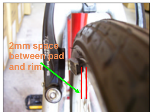
Figure 3: Brake assembly, with rim and brake pad clearance depicted.
